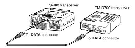
After connecting the 2 transceivers with the cable, access Menu No. 57 (DTS polarity) on the TS-480 transceiver and select "on". You will further need to adjust the audio input/ output level of the TS-480 transceiver using Menu Nos. 46 and 47.
